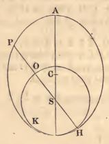
Time of fall = time of describing  $\frac{\text{circle}}{2}$  O K H, S O =  $\frac{\text{S P}}{2}$ , <u>period in the circle O K H</u> =  $\frac{\text{period in the circle rad. S O}}{\text{period in the circle rad. A C}} = \frac{\text{S O}^{\frac{3}{2}}}{\text{A C}^{\frac{3}{2}}}$
